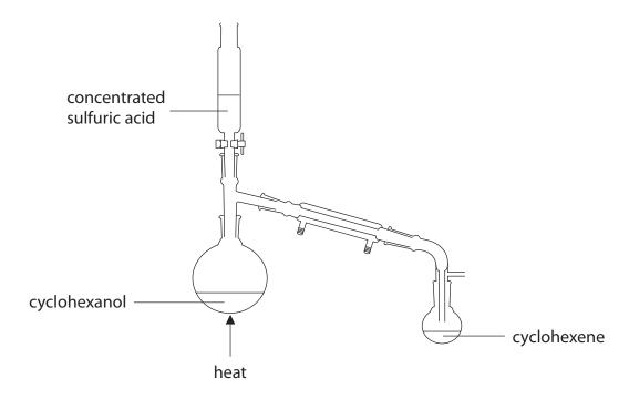
As the reaction took place, an impure liquid distilled over into the collection flask.
