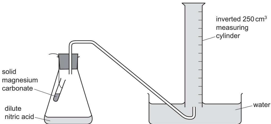
50 cm<sup>3</sup> of dilute nitric acid was added to the conical flask. The contents of the test-tube were released, allowing the solid magnesium carbonate to mix with the dilute nitric acid. A stop-clock was started and the volume of gas collected in the inverted measuring cylinder was measured every 10 seconds for 80 seconds.
