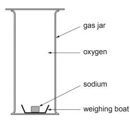
They recorded the mass of the weighing boat and its contents at the start of the experiment and then again after one week.
